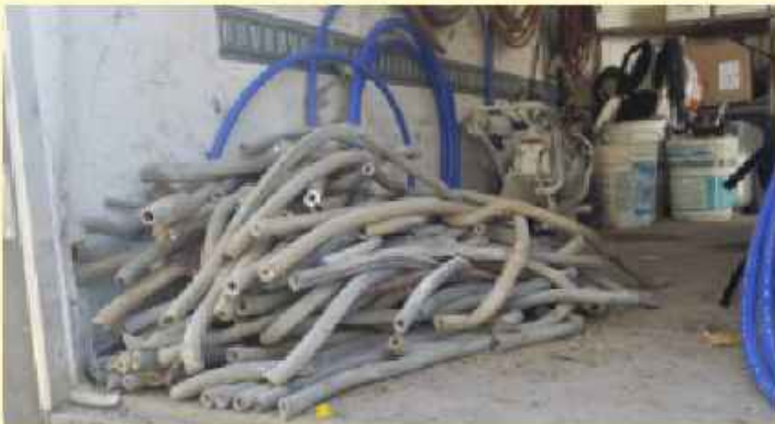
A pile of lead lines removed in Gary, Indiana. Photo: Monica Eng/Axios
